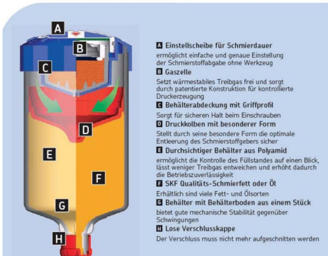
In the closed compartment the plus- minus- poles are in contact with a gel and the production of gas is activated by an electric short circuit. The amount of gas pro time unit will be regulated through an electrical resistance. The greater the resistance, the slower the production of gas. The amount of gas is proportional to the current which flows through the battery. If the supply is interrupted, the gas production will be stopped for a short period of time.
